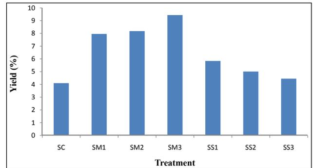
Fig. 2: Effect of pretreatments on yield of oil extracted by supercritical fluid
