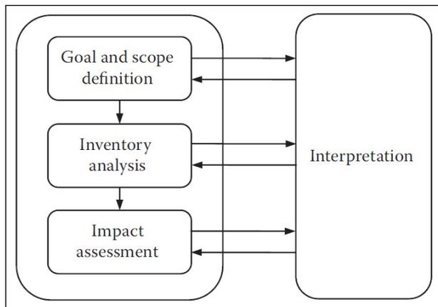
**Fig. 2:** The four iterative phases of life-cycle assessment (Jolliet *et al.* 2016)
