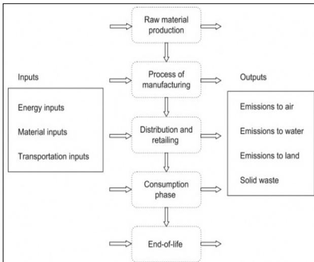
Fig. 2A: typical process flow diagram with generalized unit processes (Muthu, 2020)
